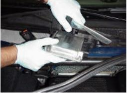
Step 9: Carefully rotate ECU and pull right wiring harness tab.
