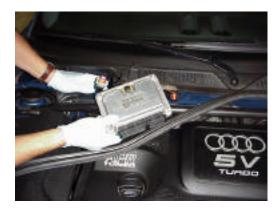
Attach electrical plugs to the ECM ensuring that the plugs are fully seated and release mechanisms are pushed all the way in.
