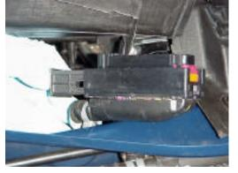
Step 7: Pry metal tab holding ECU in place with screwdriver.
