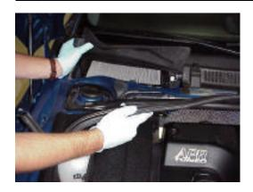
**Step 5: Remove Plastic Bracket, noting location of tabs**
