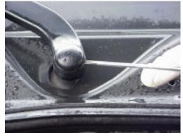
Remove Windshield Wipers to ease removal and installation of ECM.
