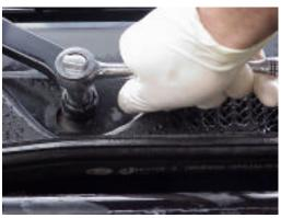
Remove the wiper arms by unbolting the 13mm nut securing the wiper arms. After the nut is removed the wiper arm must be wiggled in order to remove the arm from the mount. Be sure to note the location of the wiper arm for re-instillation.
