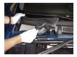
Step 6: Pull tab on wiring harness to the left, and remove left wiring harness.
